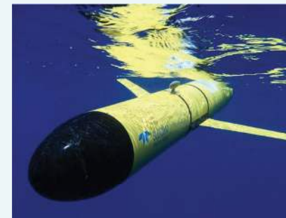
Photo: A Slocum underwater glider. Photo courtesy of Woods Hole Oceanographic Institution.
